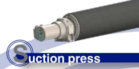
Suction presses with 1 or 2 vacuum chambers and diameters up to 1200 mm, with shells of bronze or stainless steel, able to work up to 120 kN/m pressures. We can supply the most advanced covering in the market, as per our experience.
