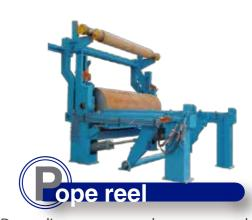
Depending on your needs, we can supply modular pope reels: semi-automatic, automatic, with or without storage of finished reel and spools. With pneumatic or hydraulic performances. The design increases efficiency of the paper production, with a spool change without production loss but with constant control of the winding
